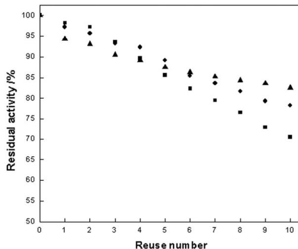
**Figure 8** Operational stability of immobilized neutral protease on (■) CS, (●) CMCS, and (▲) NSCS hydrogel beads. Enzyme activity was determined at optimum reaction conditions.
