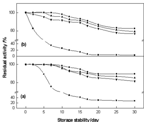
**Figure 7** Storage stability at (a) 5 and (b) 25°C of (■) free and immobilized neutral proteases on (●) CS, (▲) CMCS, and (▼) NSCS hydrogel beads. Enzyme activity was determined at optimum reaction conditions.
