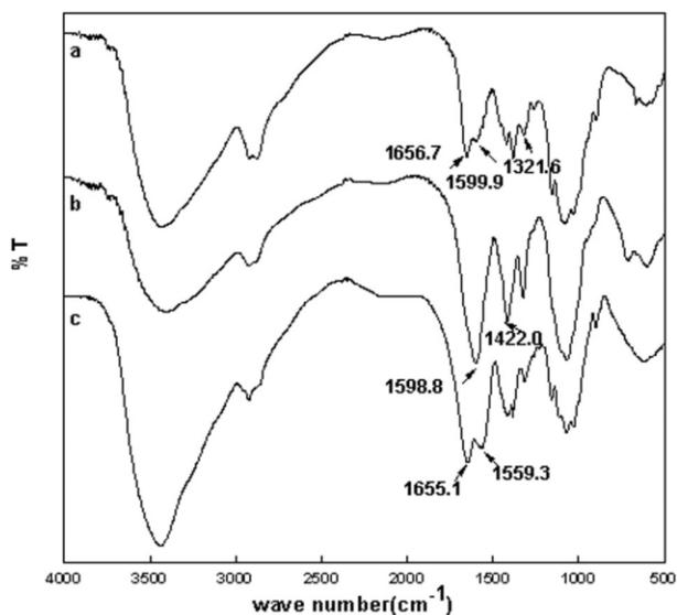
**Figure 1** FTIR of (a) CS, (b) CMCS, and (c) NSCS. % T refers to Transmittance (%).
