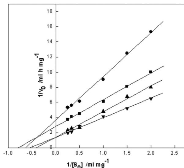
**Figure 4** Lineweaver–Burk plots for (■) free and immobilized neutral proteases on (●) CS, (▲) CMCS, and (▼) NSCS hydrogel beads. Reactions were performed at their optimum reaction conditions.  $[V_0]$  refers to initial hydrolysis rate;  $[S_0]$  refers to substrate concentration at reaction time 0.
