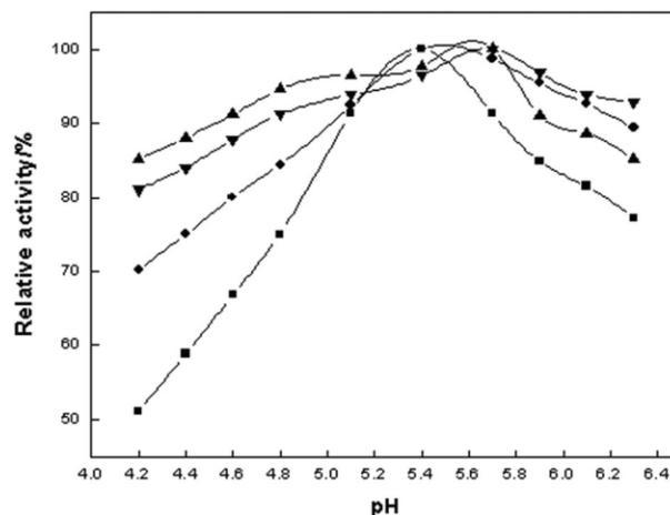
**Figure 2** Effect of reaction pH on the relatively activity of (■) free and immobilized neutral proteases on (●) CS, (▲) CMCS, and (▼) NSCS. Reactions were performed at 50°C for free and immobilized neutral proteases on NSCS beads and at 55°C for immobilized neutral protease on CS and CMCS in HAc-NaAc buffer (0.2M) of various pH values.
